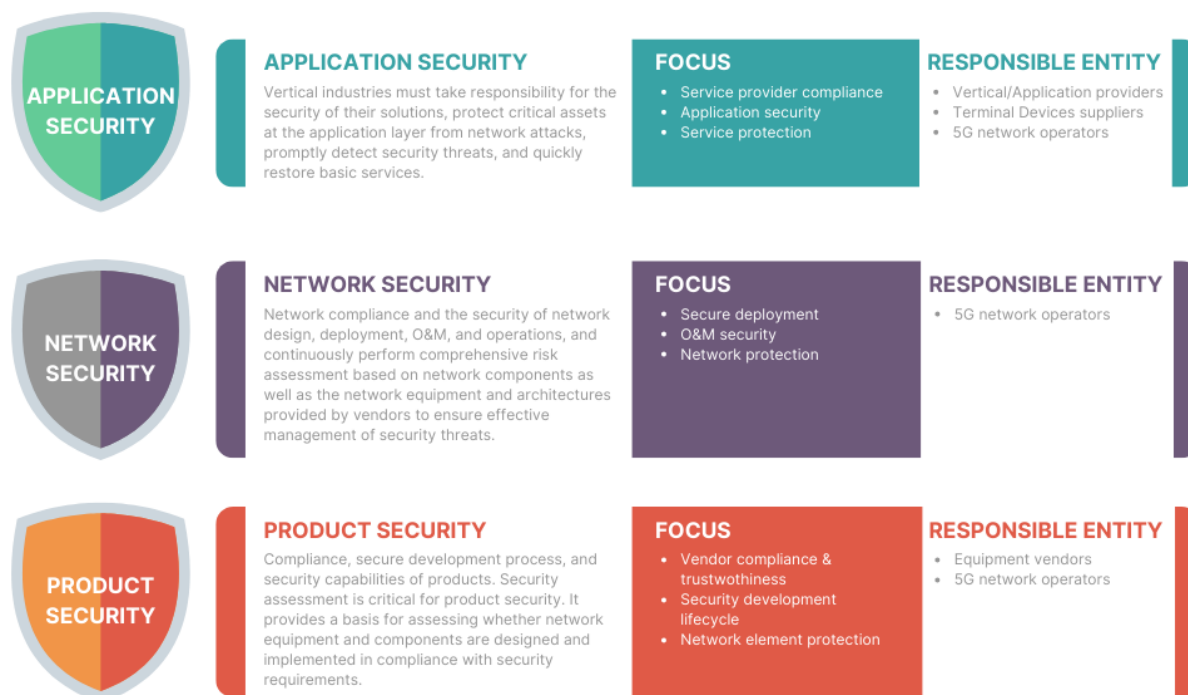
Figure-7: Three layers of the 5G cybersecurity model & responsible entities
